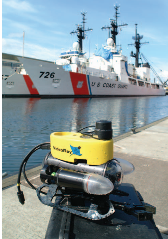
ProViewer sonar heads have been tested in concert with VideoRay portable remotely operated vehicles that have been used by U.S. Coast Guard Maritime Safety and Security Teams for conducting ship hull inspections and other operations.
