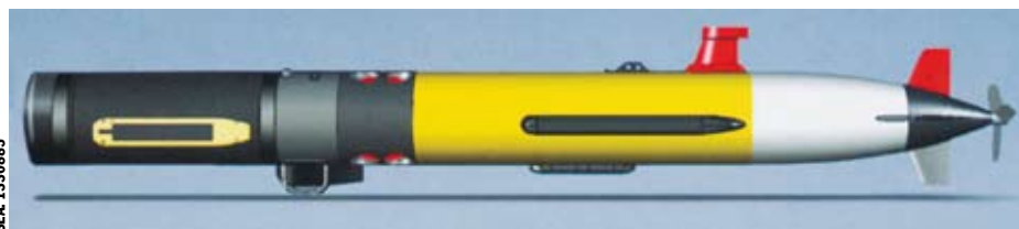
The SWATHplus-RS100 sonar fitted to the front end of the REMUS 100 UUV.
